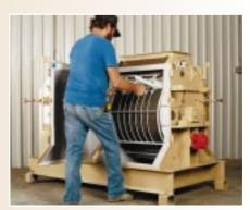
The above pictures illustrate the patented door safety locks. The hammermill rotor needs to come to a complete stop before the hammermill doors can be opened. After the doors are opened, screen change is fast, efficient and simple. One more reason why competitive manufacturers install the Bliss Eliminator Hammermill Systems into their operation.
